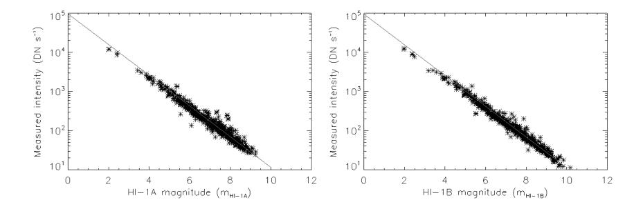
Measured stellar intensity (DN s<sup>-1</sup>) versus HI magnitude ( $m_{HI}$ ) for HI-1A (left) and HI-1B (right)
