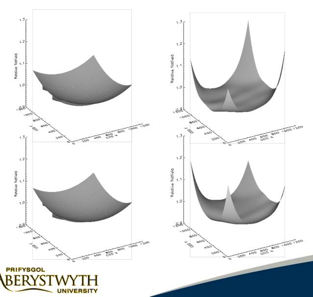
Surface plots of nominal & optimised large-scale flatfield for HI-1A (top left & right) and HI-1B (bottom left & right)
