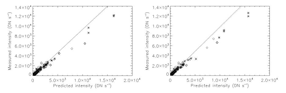
Measured stellar intensity (DN s<sup>-1</sup>) vs predicted stellar intensity (DN s<sup>-1</sup>) from spectrum folding for HI-1A (left) and HI-1B (right).
