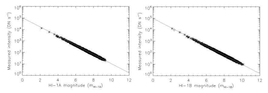
Measured stellar intensity (DN s<sup>-1</sup>) versus HI magnitude ( $m_{HI}$ ) from colour mixing for HI-1A (left) and HI-1B (right)
